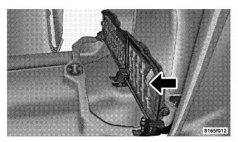
**Load Floor Securing Straps**
